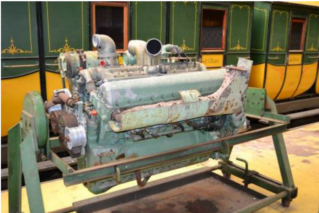
Rolls Royce tank engine
